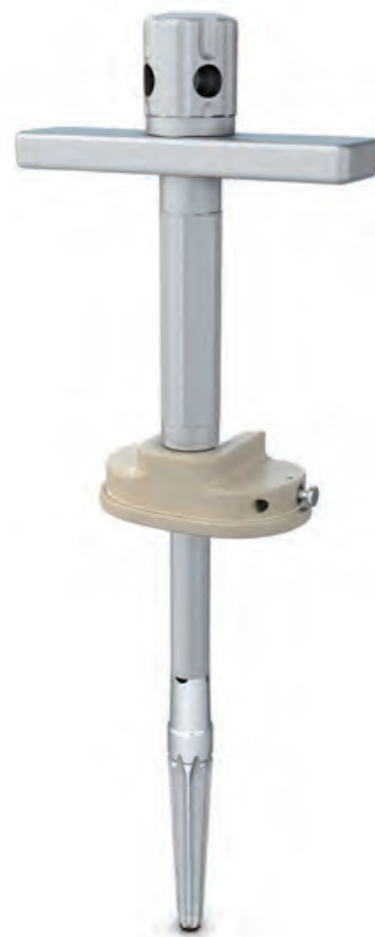
Referencing in a revision procedure (correcting a defect of about 13.5 mm with an insert height of 9 mm)
